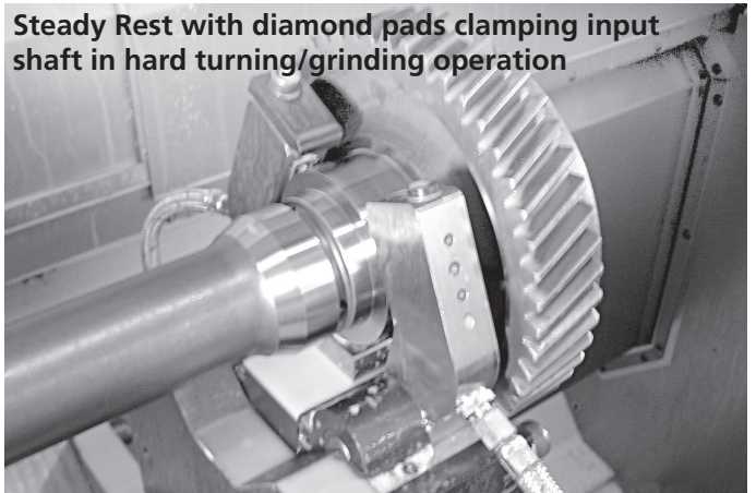
Steady Rest clamping aircraft shaft
