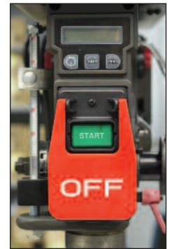
Front mount, industrial paddle on/off switch
