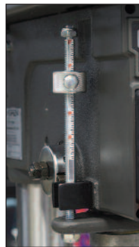
Quick change depth stop with scale
