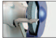
V-grooved tool rest
